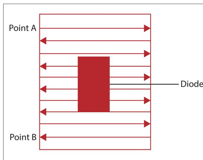
Fig. 1. Method of swabbing pulse oximeter test surface.
